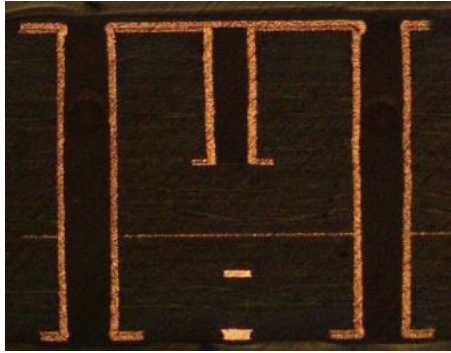
Buried blind via
